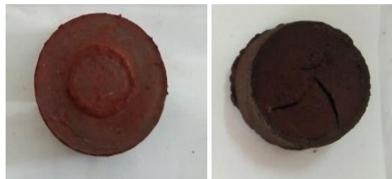
Figure 1. BaM pellet x = 0.6 (a) before sintering and (b) after sintering ( T = 1000 °C)
