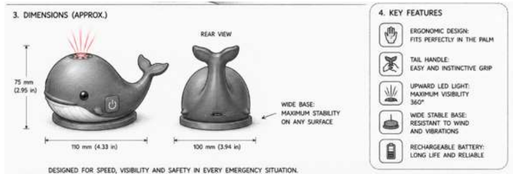
Figure 4. Possible standard dimension and functions of the device.
